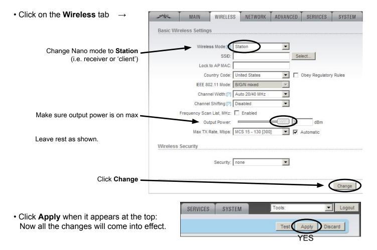
• **Note**: At this point communication with the Nano is lost because we still need to change the computers IP address to be in the same (new) range as the Nano (192.168.10.x). The setting can be either fixed (manually to e.g. IP=192 168.10.21, Subnet mask=255.255.255.0, Gateway/ Router/DNS=192 168.10.20), or **automatic** which is simpler and more flexible (as it allows you to take the computer to another wired network and automatically acquire the settings):
