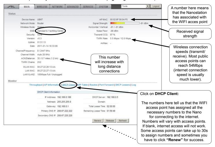
Clicking on Tools, Align antenna will bring up a received signal strength indicator, useful for improving signals by rotating the Nanostation:
